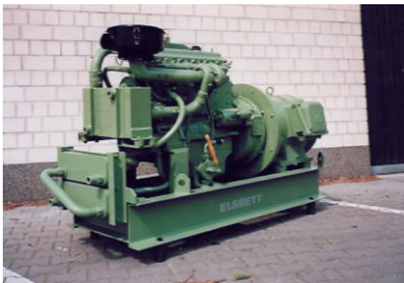
Co-generation Set 300 kW
