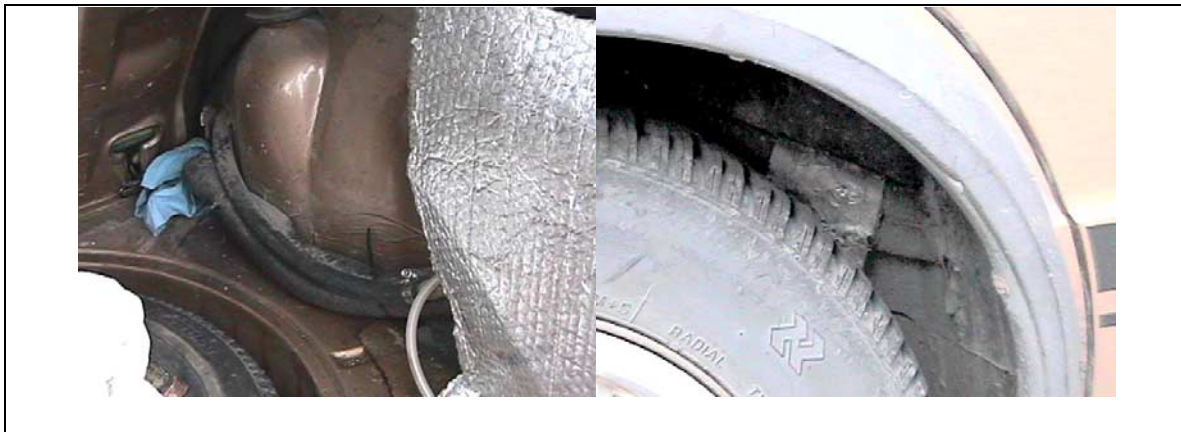
Figure 3.4 – Proof-of-Concept ROFS - HIH and Glycol Return Line Routing
