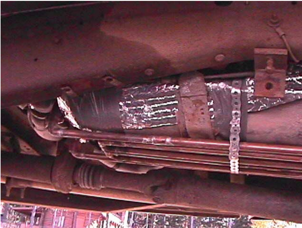
Figure 3.6 - Simplified Proof-of-Concept ROFS on Ford Truck
