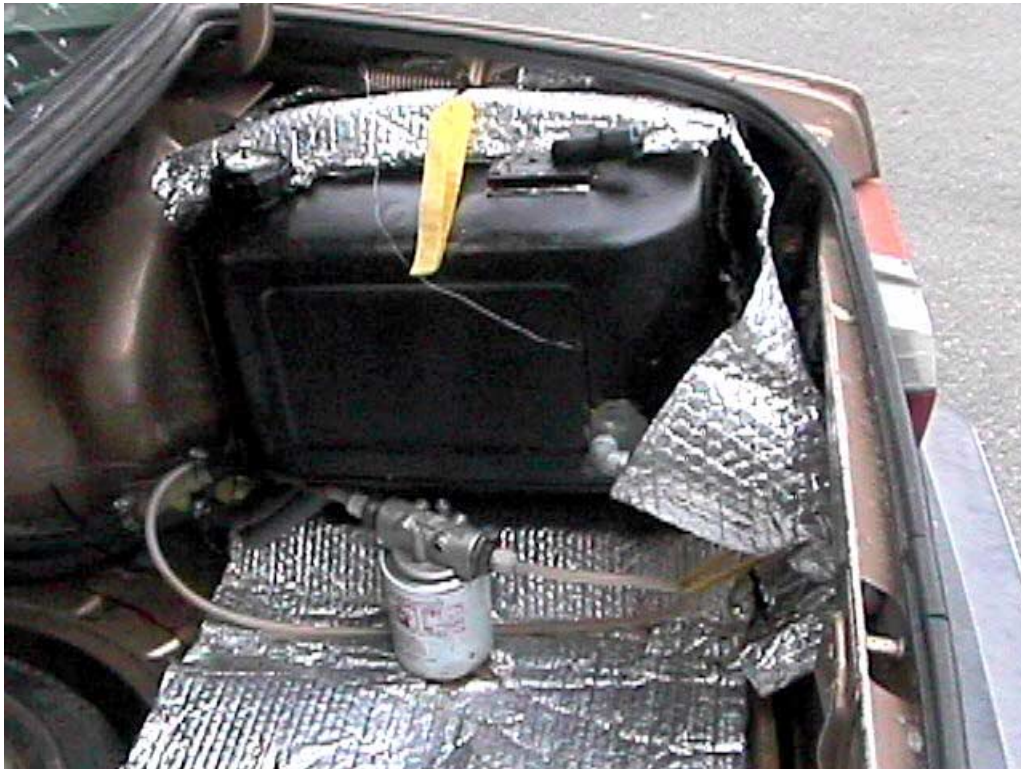
Figure 3.2 Proof-of-Concept ROFS, Auxiliary RO Fuel Tank Assembly
